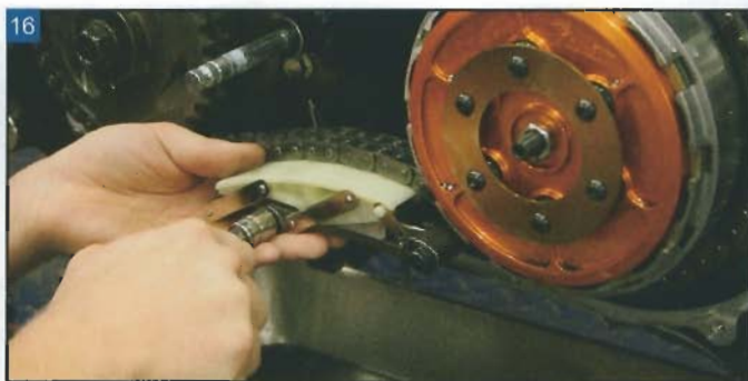
Slide the hydraulic chain tensioner into place under the primary chain.
