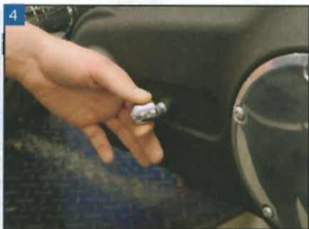
4 Loosen and remove the piece that covers the mid-shift shaft end protruding from the primary cover.
