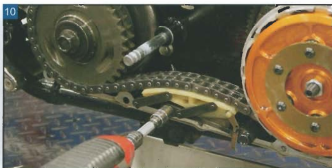
10 Loosen and remove the bolts holding the factory tensioner in place.
