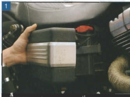
1 Remove the battery cover.
