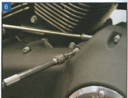
6 Loosen and remove all the outer primary cover bolts.
