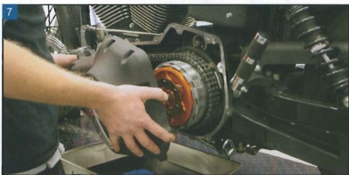
7 Remove the outer primary cover.
