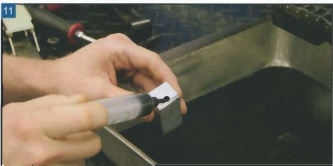
11 Using a syringe; fill the aluminum wedge block with oil per the instructions.
