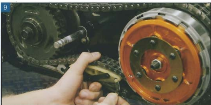
9 Squeeze the tensioner components together and put the lock in place.
