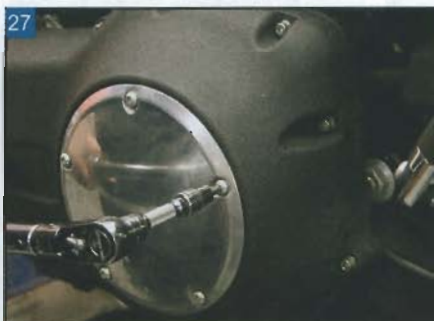
27 Replace the derby cover and tighten the bolts.
