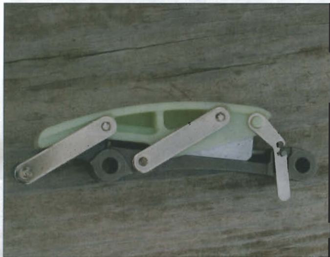
This is the HB Wedge Hydraulic Chain Tensioner from Southern Oregon Hot Bikes.
