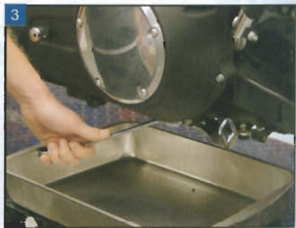
3 Loosen and remove the primary chain case drain plug.
