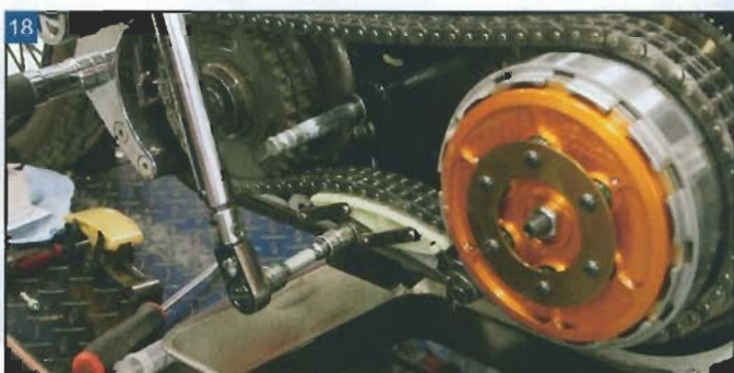
Torque the bolts to the factory specifications.
