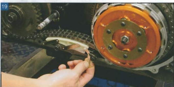
Remove the locking clip.
