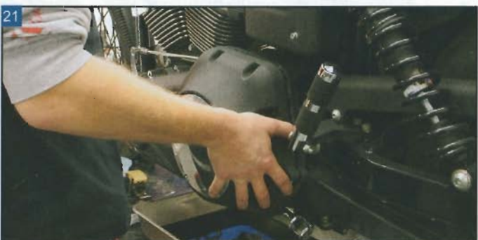
Reinstall the outer primary cover.
