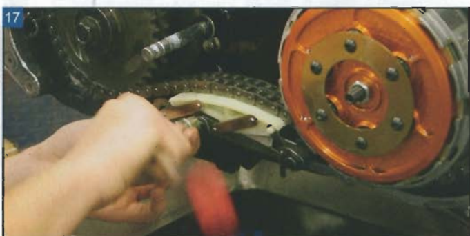
Tighten both chain tensioner bolts at this time.
