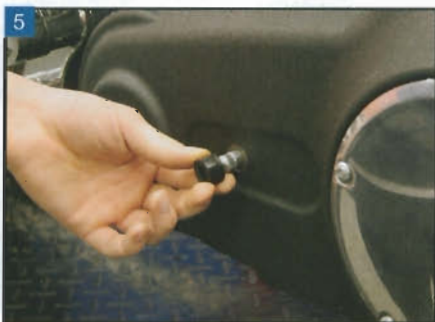
5 Remove the rubber spacer.
