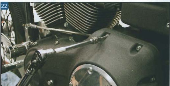
Install and tighten the outer primary cover bolts.
