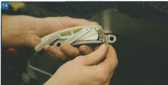
14 Squeeze the hydraulic chain tensioner together and place the locking clip on the tab to keep it compressed.
