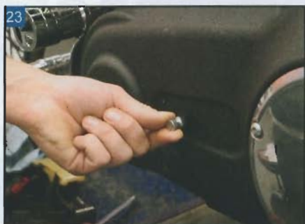
23 Reinstall the rubber spacer on the mid-shift shaft.
