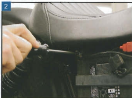
2 Disconnect the battery for safety.
