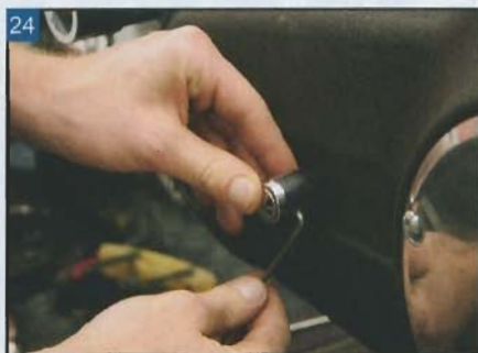
24 Reinstall the shaft-end cover and tighten the allen-head bolt.
