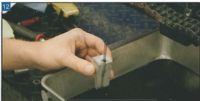
12 Place the long spring into the wedge block.
