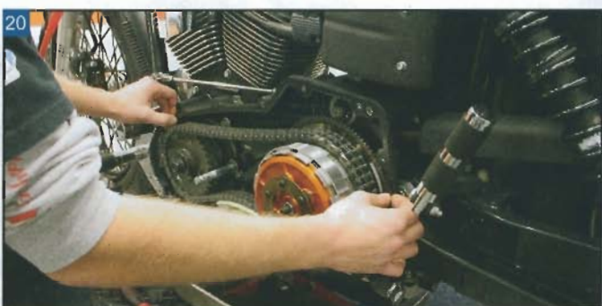
Install a new primary chain case gasket.
