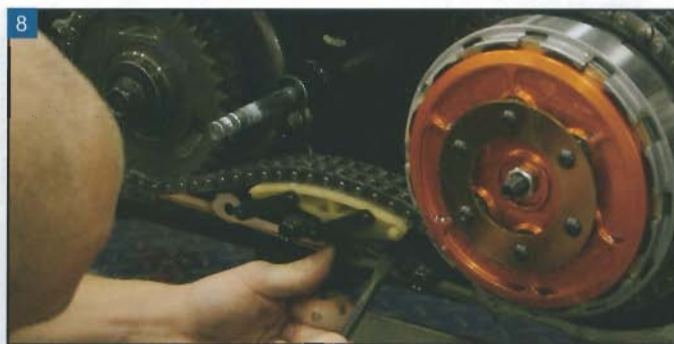
8 Release the spring-loaded chain tensioner.
