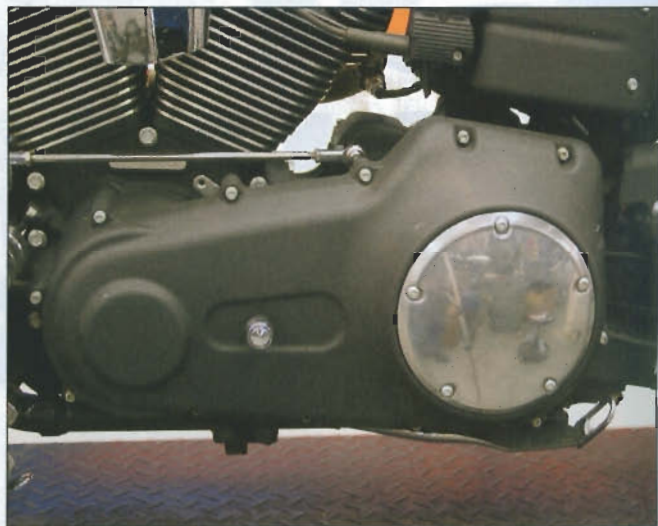
This '07 Harley-Davidson® Street Bob (Dyna Glide) will have its existing primary drive chain tensioner replaced with the hydraulic unit from SOHB.
