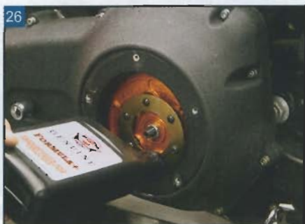
26 Install the chain case drain plug and fill the primary chain case with lubricant.
