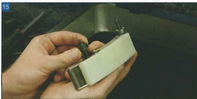
Slide the bolts through the hydraulic chain tensioner and put the spacers on the backside.
